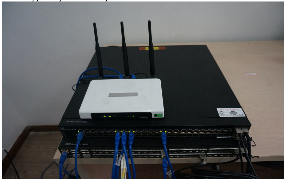
Figure 7 OpenFlow-enabled switches and wireless router (Top to down: TP-LINK TL-WR1043ND, IBM G8052, and IBM G8264)
