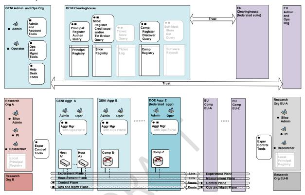
Figure 2-2. System Diagram with Federated Infrastructure Suites.
