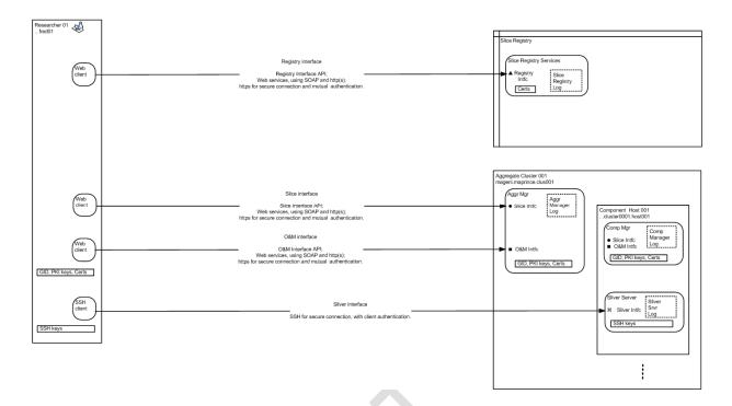
Figure 4.3 – Researcher to Registry and Aggregate Message Flows (Changes required in figure)
