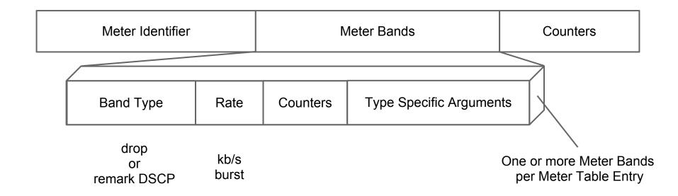
"the meter applies the meter band with the highest configured rate that is lower than the current measured rate"
