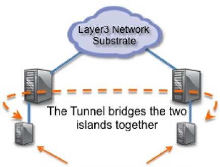
Br2 interface on both hosts cannot reach either side until the GRE tunnel is brought up
