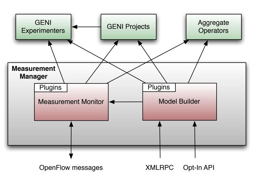
The Measurement Manager consists of two main components, a Model builder to construct a model of the OpenFlow aggregates; and the Measurement Monitor which collects information by becoming an OpenFlow controller and monitoring all controller traffic from the OpenFlow enabled devices.
