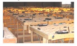
All of the arrays are organized in a grid which is deployed approximately 3 feet off the ground, by using an array of wooden tables. The configuration of the grid is as follows.
