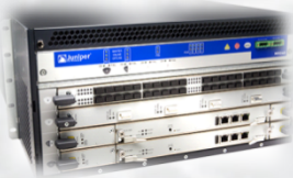
Juniper MX240 Ethernet Services Router
