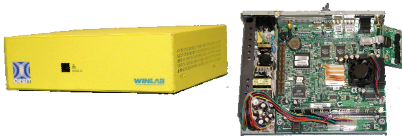
ORBIT Multi-Radio Node (v1.0) with integrated Chassis Manager
