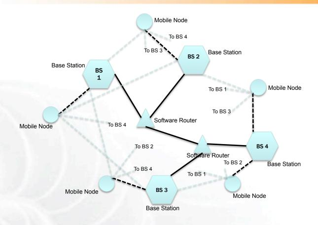
Base stations connected by a high-speed wired network Mobile nodes have physical links to all base stations But only one link is active (based on computed signal strengths) – simulates RF link between mobile device and base station
