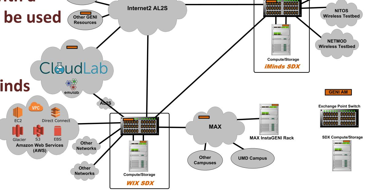
• Distributed SDX infrastructure can be used for "per-flow" value added processing, or to build specialized service topologies
