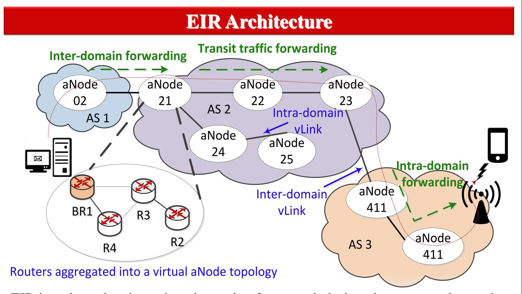
• EIR is a clean slate inter-domain routing framework designed to support the needs of mobile wireless access at the edge
