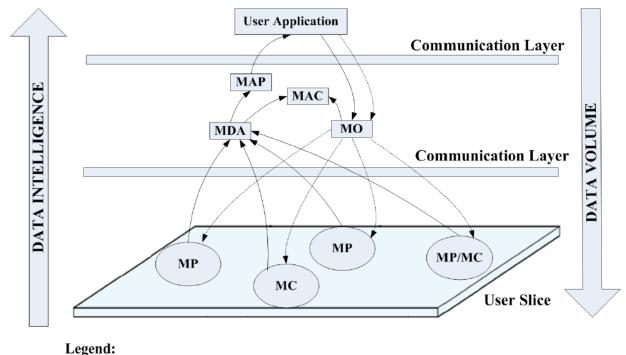
**Data Flow** MDA - Measurement Data Archive **Control Flow** MO - Measurement Orchestration MAC - Measurement Access Control Measurement Point
