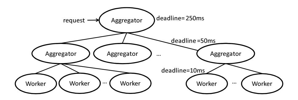
Partition/aggregate pattern Alizadeh et al., "Data center TCP", SIGCOMM' 10
