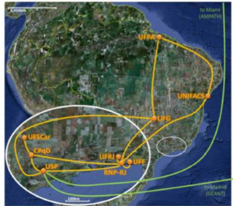
Expected topology of interconnecting private L2 network and alternatives for BR-EU link
