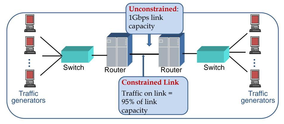
Laboratory **testbed** for experiments
