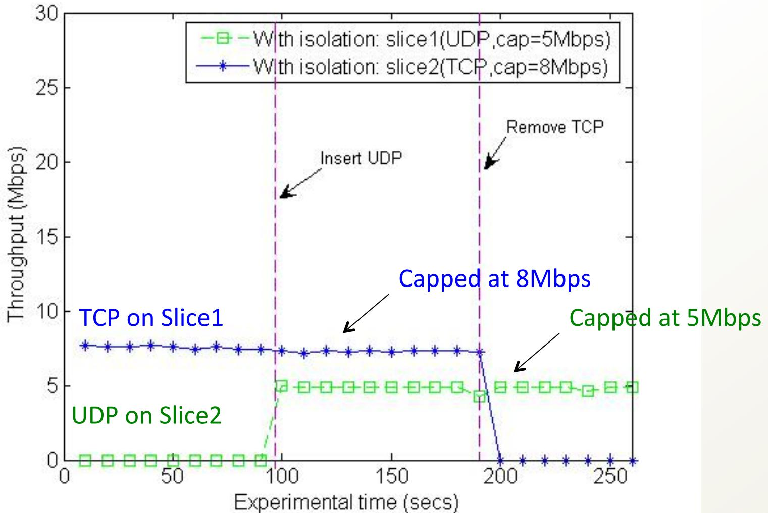
→ TCP flow on Slice1 and UDP flow on Slice2 are BW-capped
