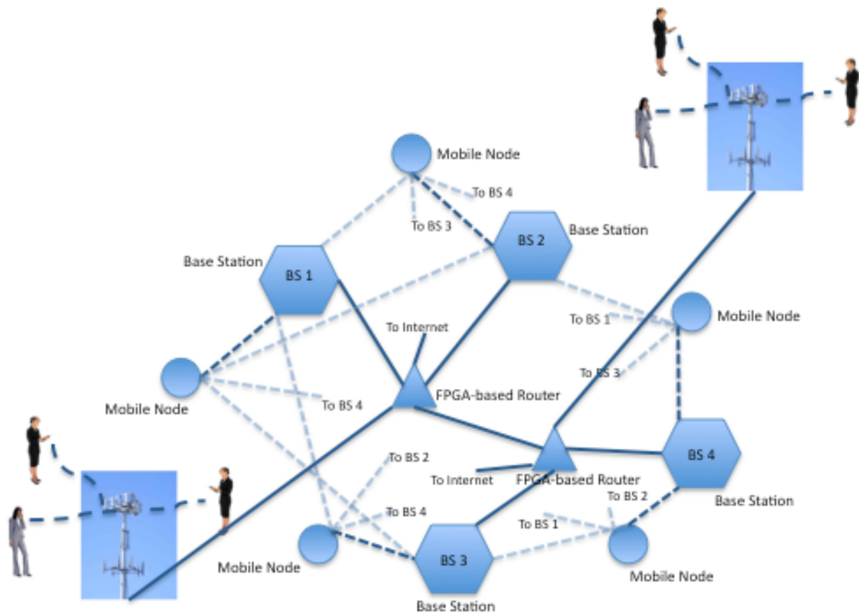
Figure 4. Experiment network configuration with real base stations and opt-in users.
