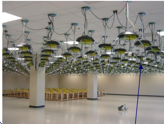
400-node Radio Grid Facility at WINLAB Tech Center
